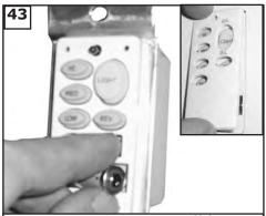
Remove cover by snaping off from top or bottom. Install 12V battery into wall remote. Duracell MN21 / Eveready A23 / GP 23A all 12V.
